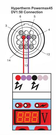
While being a universal THC, accepting full raw arc voltage for most any plasma cutter on the market, an exciting new standard feature of this unit is the addition of a 1:50 divider for an extremely fast, simple installation on most major brands. There will most likely be a direct connection for this on the outside of the plasma cutter's unit. Please refer to your plasma cutter owner's manual.
