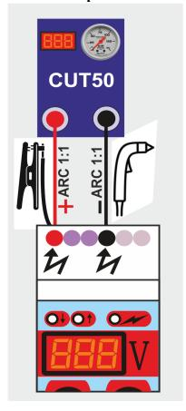
**ATTENTION**: When connecting directly, use the shortest possible cables for connecting the plasma source with THC controller - it is recommended the THC controller to be located directly at the plasma source.
